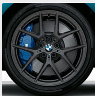
□ 18" M light alloy wheels V-spoke style 554 M Orbit Grey metallic, 8J x 18 with 225/40 R18 tyres. 3,*
