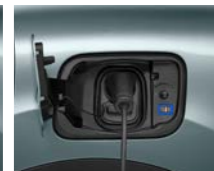
Deferred Charge Mode (Flashing blue LED)
