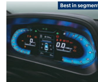
Digital cluster with TFT multi information display (MID)
