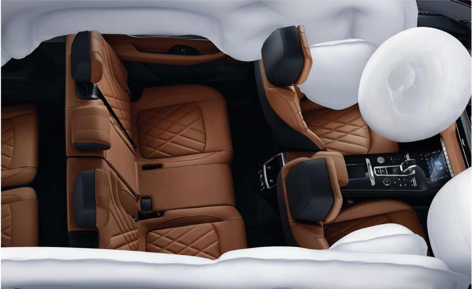
The **Tiggo 8 pro** is equipped with guard-ring type 6 airbags to provide full protection in event of collision. It has front and side airbags for the driver and front passenger as well as overlong side curtain airbags to protect the cabin's interior.
