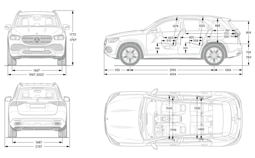
At minimum to maximum height with steel suspension. All figures in millimetres. The illustrated dimensions are averages. They are valid for vehicles in basic specification and in unladen condition.
